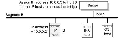
Figure 6-3 Assigning an IP Address to the Entire Bridge
